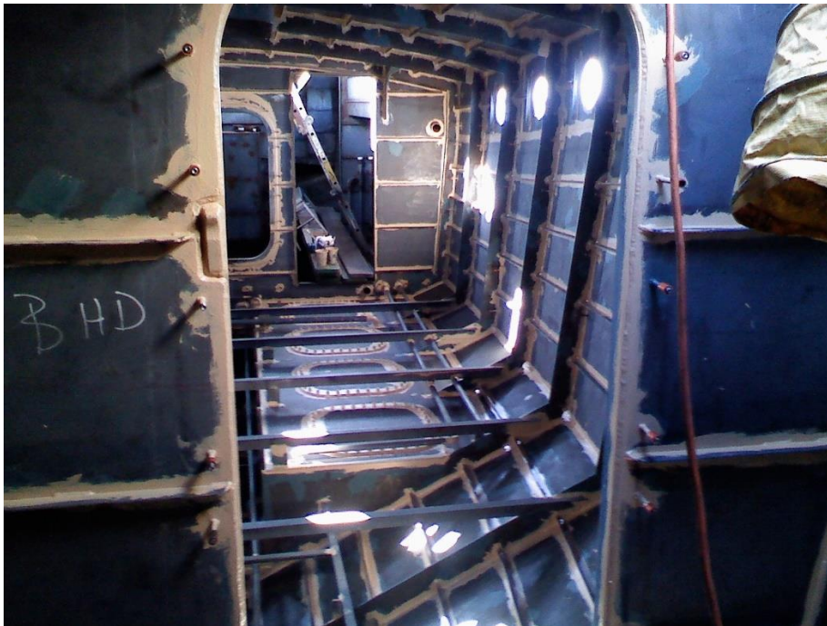
This is what proper strip coating looks like. An extra layer of paint on every edge and every joint.
